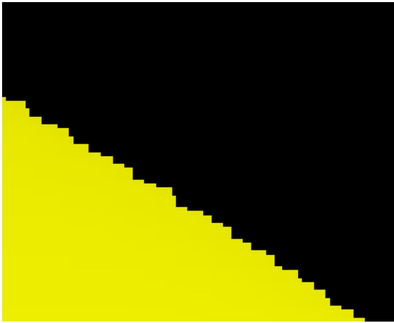
Figure 1: Close-up of a sphere rendered with one ray per pixel
